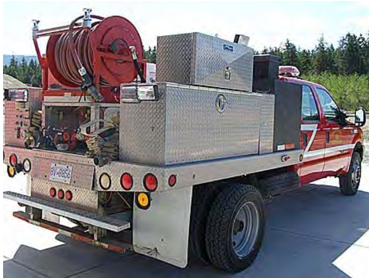
Photo 1 Dashwood Volunteer Fire Department wildland fire truck (2001 Ford F550: 350 gallon water tank, 5 gallon foam tank). This is a specialised unit to deal with wildland fires
